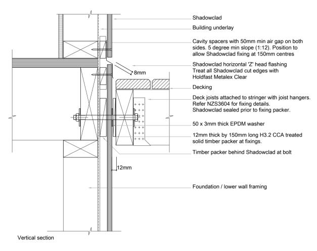
SC048 Shadowclad Mid floor to Non-Cantilevered Deck (Cavity)
