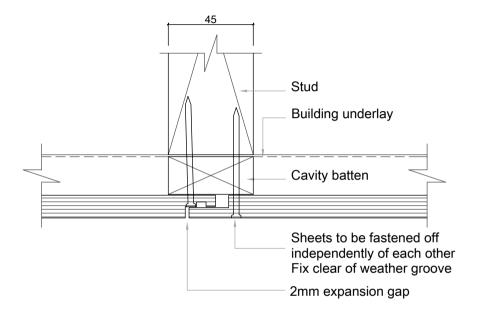
SC006 Shadowclad Texture Vertical Joint (Cavity)
