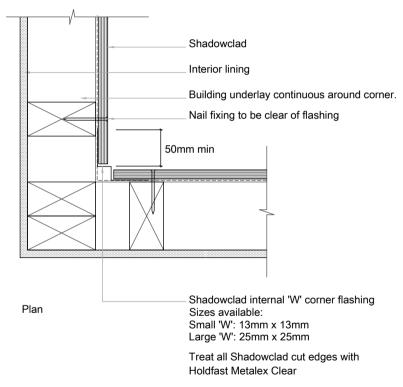
SC025 Shadowclad Internal Corner w/ W Flashing (Direct)
