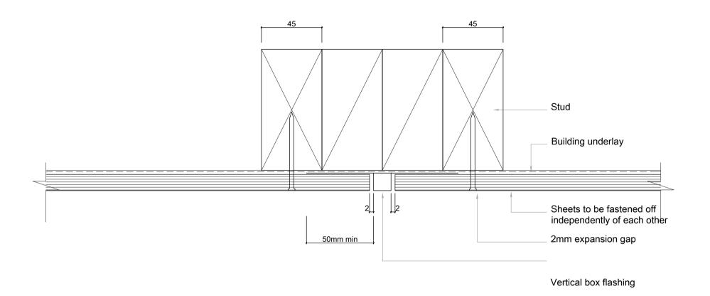
SC013 Shadowclad Vertical Joint with Top Hat Flashing (Direct)
