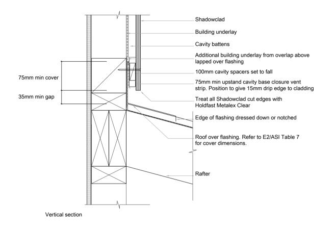
SC050 Shadowclad Basic Apron Flashing (Cavity)
