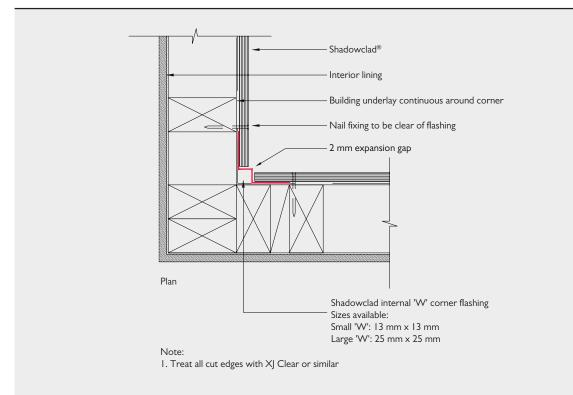
Flashings should have expansion joints where necessary to provide adequate allowance for thermal expansion as set out below.
