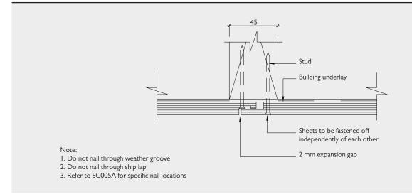
SC005A: Shadowclad Texture Vertical Joint Fastener Locations (Direct Fix)
