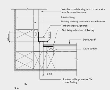
I. Allow 2 mm expansion gap between flashing and cladding
