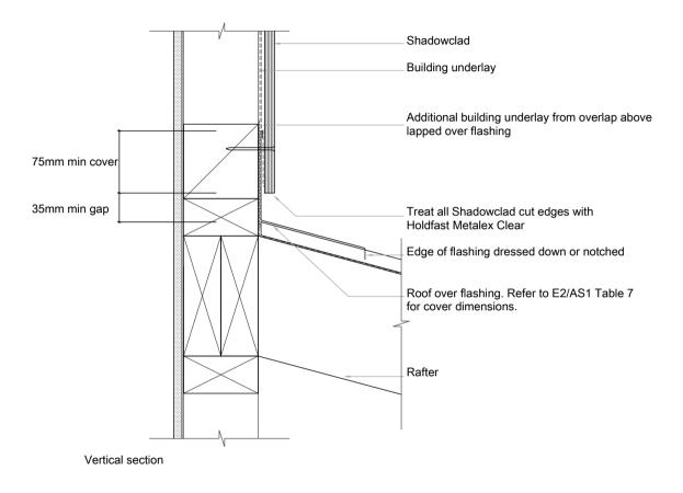
SC049 Shadowclad Basic Apron Flashing (Direct)
