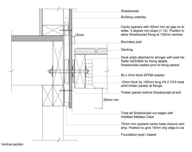
SC046 Shadowclad Timber Ground Floor to Non-Cantilevered Deck (Cavity)
