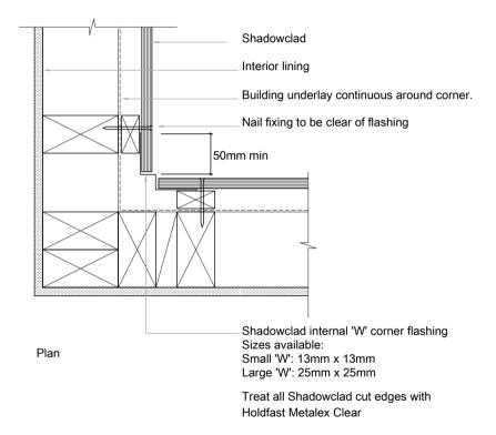
SC026 Shadowclad Internal Corner w/ W Flashing (Cavity)
