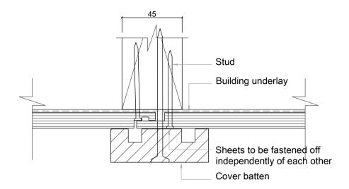
SC009 Shadowclad Vertical Joint option cover batten (Direct)
