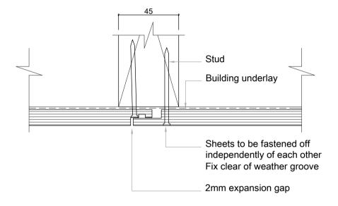
SC005 Shadowclad Texture Vertical Joint (Direct)
