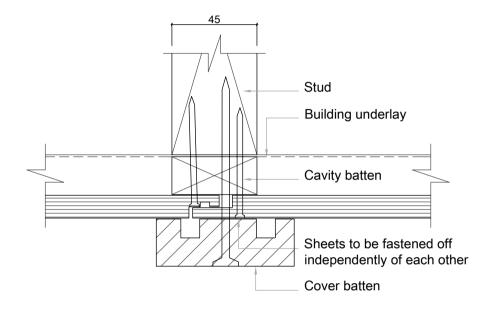
SC010 Shadowclad Vertical Joint option cover batten (Cavity)
