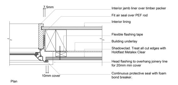
SC030 Shadowclad Jamb detail (Cavity)
